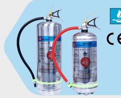
WET CHEMICAL (K-CLASS) TYPE KITCHEN FIRE EXTINGUISHER OFFER AN DISTINCTIVE UNIQUE FEATURE BY REACTING CHEMICALLY WITH COOKING OIL OR FATS (SAPONIFICATION) & FORMS A NON-COMBUSTIBLE LAYER ON SURFACE, THEREBY PROVIDES A VERY FAST FLAME KNOCK DOWN & COMPLETE SECUREMENT OF GREASE RELATED FIRES. AVAILABLE IN STAINLESS STEEL CYLINDERS AND MILD STEEL CYLINDERS
